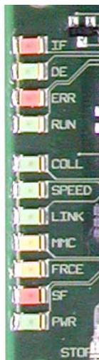
On the plug-in module you can see a LED bar for status monitoring of the CPU and the Profibus DP master. Especially at the commissioning and the external usage of the module, the state of your CPU and your Profibus-DP master is shown.
