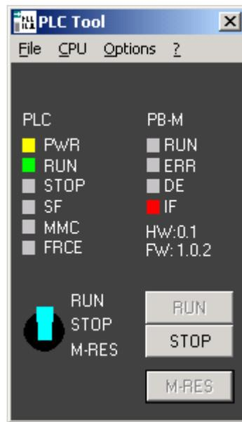
The operating surface (see figure above), which is a schematically top view of a CPU, serves for monitoring and operating the CPU. Here, the status of the LEDs on the CPU as well as the position of the mode switch are shown.
