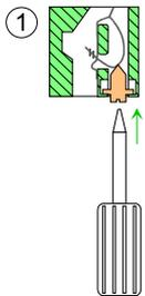
For the cabling of power supply of a CPU, a green plug with CageClamp technology is deployed.
