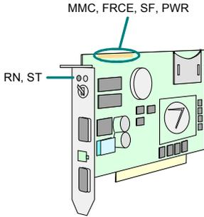
1. Get the RUN-STOP lever of your CPU in position STOP. Turn off the voltage supply. In installed condition depending upon operating system now you get a message that the connected partner is no longer present. This message can be ignored. Plug the MMC with the firmware files into the CPU. Please take care of the correct plug-in direction of the MMC. Turn on the voltage supply.
